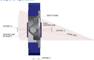
The combination of these three offsets provides an uninterrupted sealing surface, whilst maintaining sealing integrity over the valves lifecycle with minimised wear between the seat and seal. The conical profile on both the seal stack and the seat face ensures there is no seal/seat contact during operation, limiting flow induced wear in this area. The optimised seating angle can minimise binding of the disc and in doing so reduces required operational torque.
