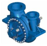
Radially split, single stage, double suction, between bearings Capacity: 53,000 gpm / 12,000 m<sup>3</sup>/h Head: 1,250 ft / 380 m Pressure: 1,450 psig / 100 bar Temp Range: -22°F (-30° C) to 850° F (455° C) Speed: 3,600 rpm
