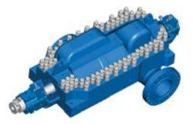
Axially split, volute or diffuser, single or double suction, between bearings Capacity: 8,800 gpm / 2,000 m<sup>3</sup>/h Head: 8,200 ft / 2,500 m Pressure: 2,175 psig / 150 bar Temp Range: -22°F (-30° C) to 390° F (200° C) Speed: 3,600 rpm
