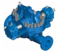
Axially split, single and two stage, double suction, between bearings Capacity: 53,000 gpm / 12,000 m<sup>3</sup>/h Head: 2,500 ft / 760 m Pressure: 870 psig / 60 bar Temp Range: -22° F (-30° C) to 390° F (200° C) Speed: 3,600 rpm
