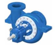
Centerline mounted, single-stage, overhung Capacity: 11,000 gpm / 2,500 m<sup>3</sup>/h Head: 1,250 ft / 380 m Pressure: 3,045 psig / 210 bar Temp Range: -150°F (-100° C) to 850° F (450° C) Speed: 3,600 rpm
