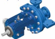
Centerline mounted, single-stage, low flow Barske type Capacity: 65 gpm / 15 m<sup>3</sup>/h Head: 656 ft / 200 m Pressure: 580 psig / 40 bar Temp Range: -150°F (-100° C) to 850° F (450° C) Speed: 3,600 rpm
