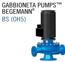
Vertical in-line, single-stage, close coupled, overhung Capacity: 2,200 gpm / 500 m<sup>3</sup>/h Head: 1,000 ft / 300 m Pressure: 928 psig / 64 bar **Temp Range:** -40°F (-40° C) to 480° F (250° C) Speed: 3,600 rpm
