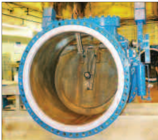
Compressor Check Valve with Oil Dashpot
