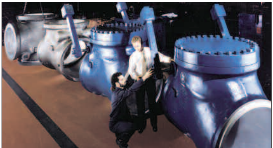
44" Cold Reheat Check Valves
