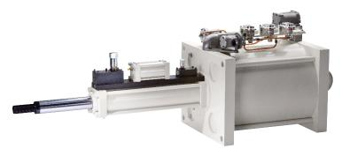
Tandem linear pneumatic actuators include all the features of our linear pneumatic actuators with the addition of a hydraulic cylinder to facilitate precise and repeatable speed control.
