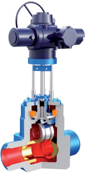
The highly versatile Hopkinsons® Flexi-Wedge Design of gate valve is designed for containment isolation duties in the nuclear industry where a wedge gate valve is the preferred design option. The wedge gate valve seals by using mechanical force. Closure is achieved by applying a downward force to the wedge to seal on both tapered seats. The seat faces are self centering which ensures consistent closure through the lift of the valve.
