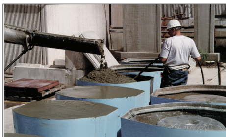
Step 5: Multiple shells may be filled simultaneously.
